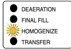
10. During **HOMOGENIZE** Operation, the mixer motor will stir the solution for ten (10) minutes. When the HOMOGENIZE Operation is complete, the Transfer Indicator Light will flash. Remove Large Access Lid and look into the tank to make sure the granules have dissolved and the solution is colorless. Once you have verified the granules are dissolved and colorless, the solution is ready for Specific Gravity Testing.
