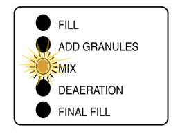
For the **99 Gallon Dry Acid Dissolution Unit**, during the **MIX** Operation, the solution is mixed for a period of thirty-five **(35) minutes** allowing the granules to completely dissolve. The Dry Acid Dissolution Unit will then automatically step to the DEAERATION Operation.
