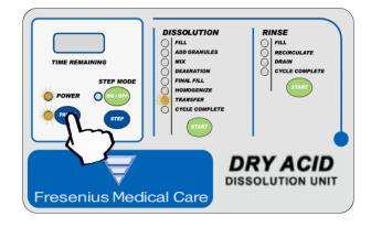
When the Dry Acid Dissolution Unit is empty, the Dry Acid Dissolution Unit will step to the CYCLE COMPLETE Operation.
