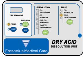
Recirculate Operation will stop and DRAIN Valve will open.
