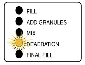
For the 99 Gallon Dry Acid Dissolution Unit, the DEAERATION Operation runs for two (2) minutes during which the entrapped air is allowed to separate out of the solution. Upon completion, the Dry Acid Dissolution Unit will automatically step to FINAL FILL Operation and the Final Fill Indicator Light will illuminate.
